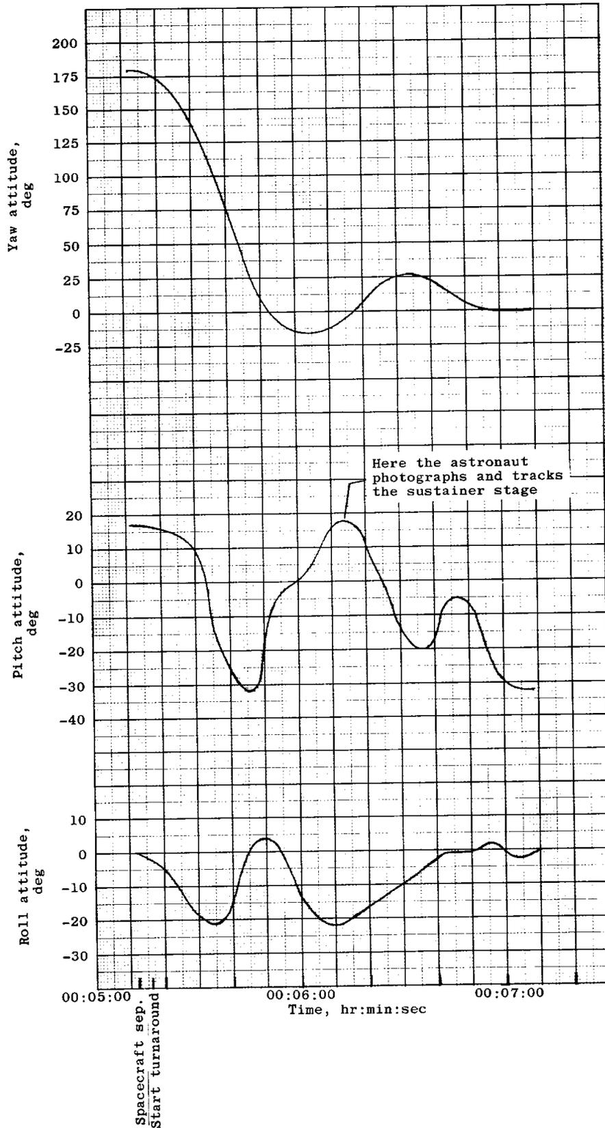
Figure 7.2.3.1-1.- Turnaround maneuver; fly-by-wire control mode, rate and attitude gyro indicator.
