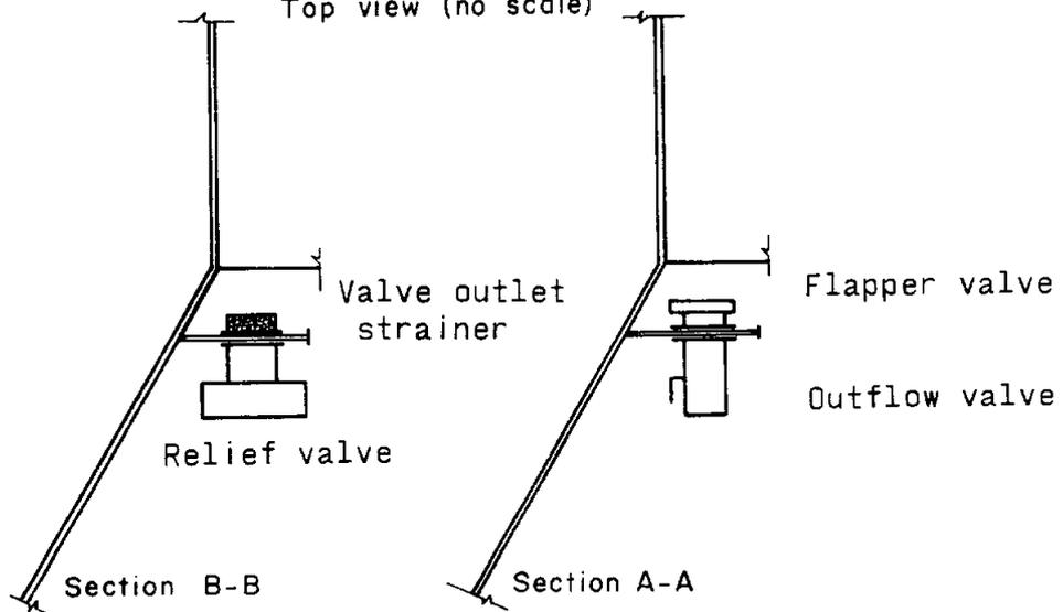
Figure 5.5.7-1.- Sketch showing location of valves in spacecraft small pressure bulkhead.
