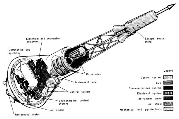
FIGURE 1-1.—Spacecraft interior arrangement.
