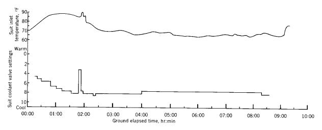
FIGURE 1-6.—Suit-inlet temperature and coolant-control-valve setting.
