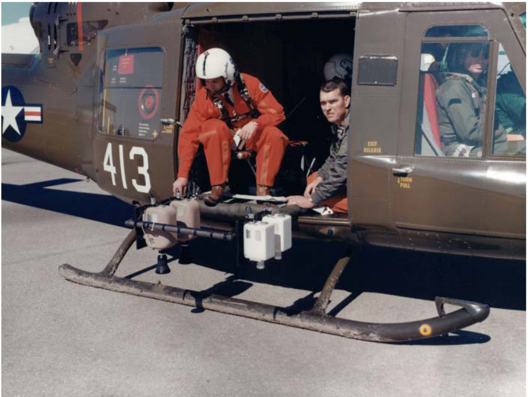
Photo 16 Mounted cameras on one of the pickup helicopters
