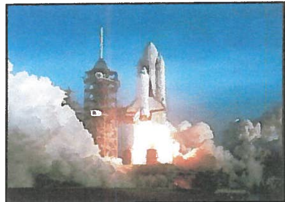
The external tank was painted white for the first two shuttle launches. From STS-3 on, it was left unpainted.
