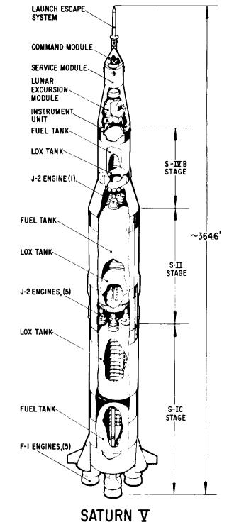
AS TALL as a 35-story building and as heavy as two dozen big jet transports — that's the Saturn V/ Apollo Moon vehicle under construction by the NASA-Marshall Space Flight Center, Huntsville, Ala. This new drawing shows the various elements of the big vehicle which is 375 feet tall with a maximum diameter of 33 feet.
