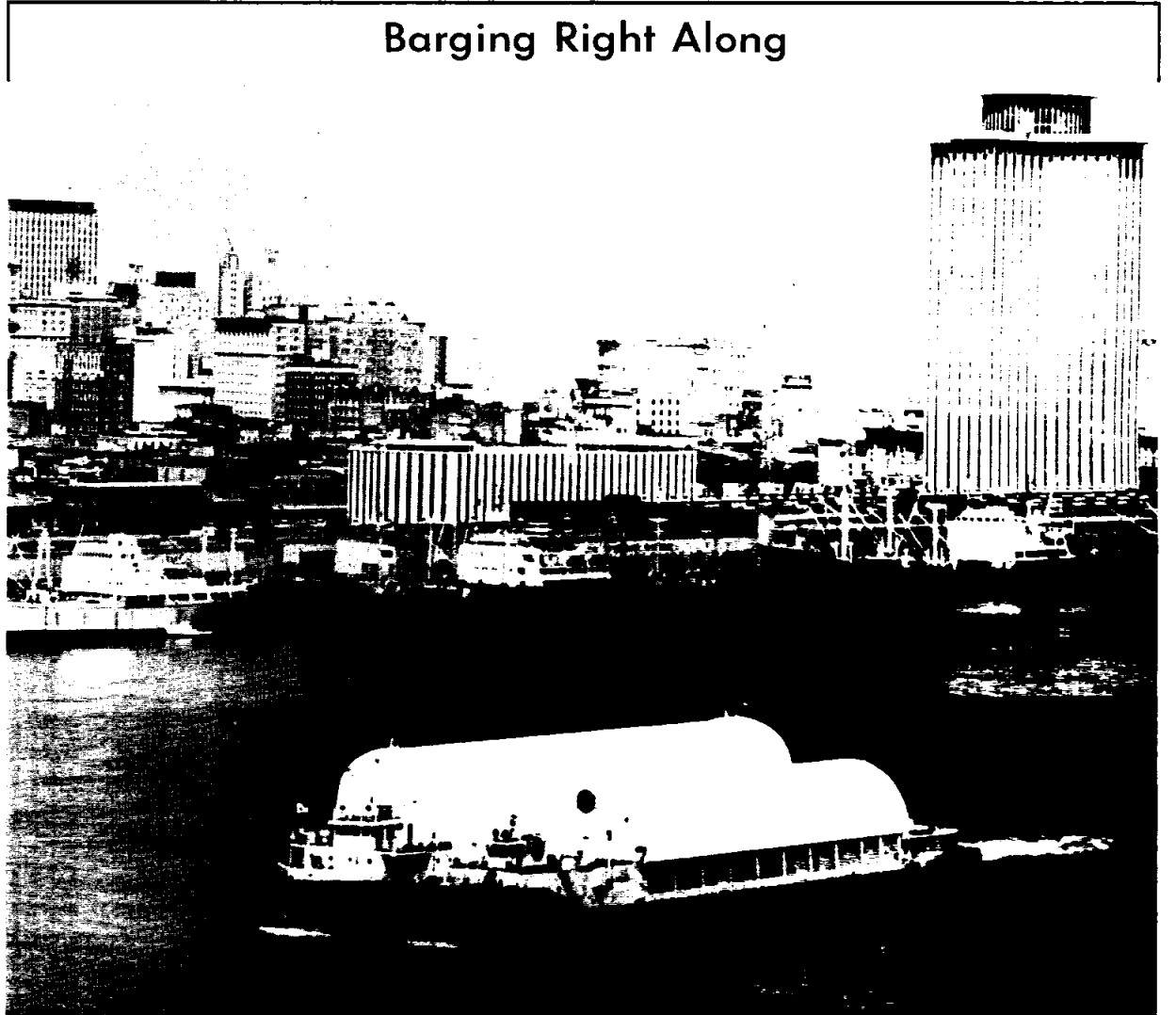
SATURN FERRY —Two NASA barges carrying first stages of Saturn V and uprated Saturn I pass the New Orleans skyline after leaving NASA's Michoud Assembly Facility. The Poseidon , on the left, carries the first flight version of Saturn V to Marshall Space Flight Center for static firing. The Promise returns an uprated Saturn I ground test vehicle to Marshall. The 1000-mile trip up the Mississippi, Ohio and Tennessee rivers requires about eight days.
