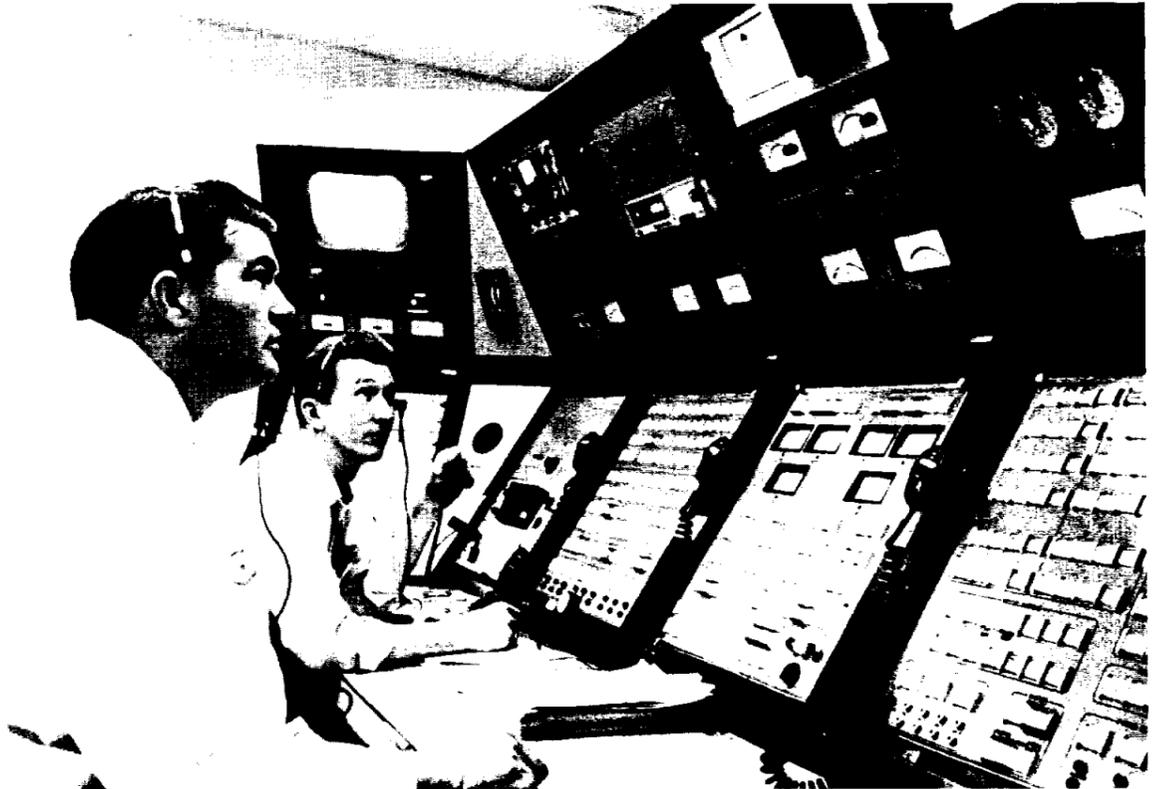
**BEHIND THICK WALLS**—Don Lotspeich of BR-N, left, and Bill Taliaferro of Thermochemical Test Branch monitor Apollo service module RCS thruster quad firings at the control panel in the Auxiliary Propulsion Test Facility. Closed-circuit television monitors show the thrusters in the 20-foot diameter subsystem test vacuum chamber. The control room is separated from the test chamber by foot-thick reinforced concrete walls.
