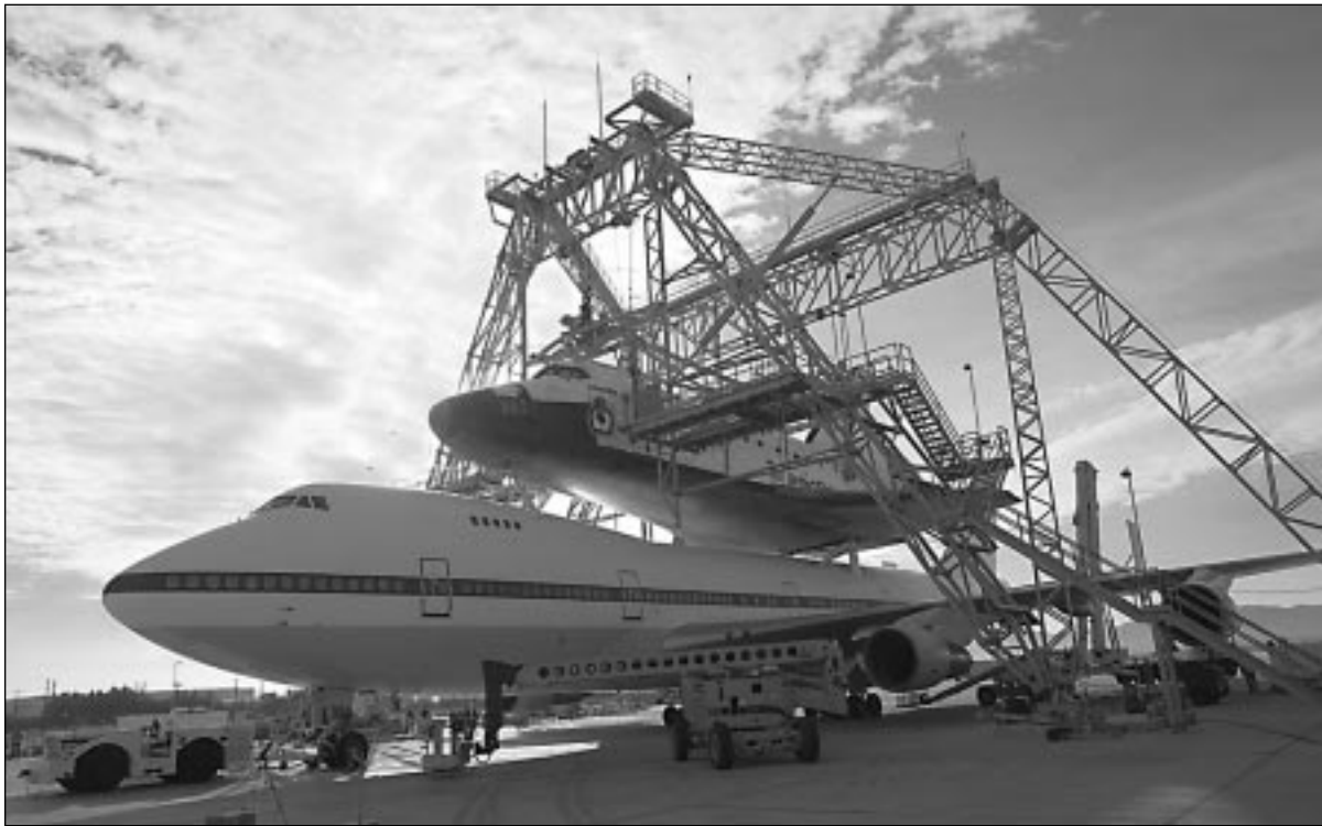
Above: Technicians prepare to lift Atlantis off of its Shuttle Carrier Aircraft following a November ferry flight from Kennedy Space Center to Palmdale, Calif. Right: Manufacturing engineer Darrell Trojan, center, meets with members of his Palmdale, Calif., major modification team. Below: Mark Allison, a Boeing employee, examines the flight deck of Atlantis . The cockpit will change significantly during this major modification period with the installation of "glass cockpit" liquid crystal displays to replace the old mechanical cockpit displays.
