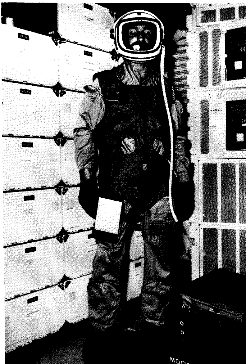
Integrated Harness Restraint, Launch and Entry Helmet, and Personal Egress Air Pack
