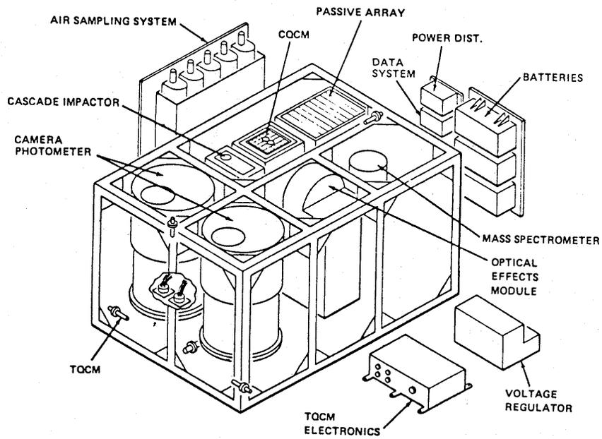
With the monitor instrumentation, contaminant sources are identified for possible elimination. The experiment provides data on the interaction of the induced and natural environments, and provides critical data for planning of future Shuttle payloads.
