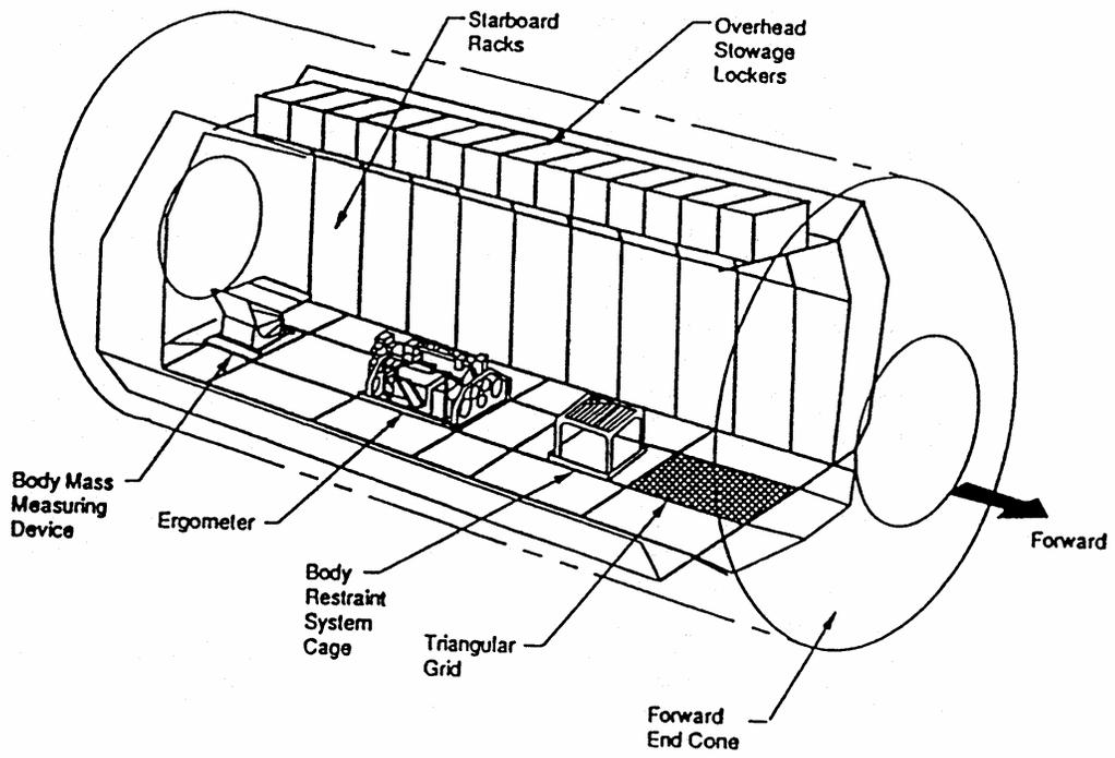
SLS-2 module isometric view
