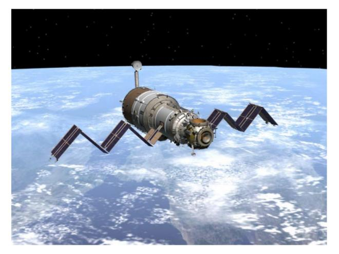
At about the same time, Zvezda's solar arrays are to deploy and immediately begin following the sun; meanwhile, automatic commands will order the activation of the module's major systems
