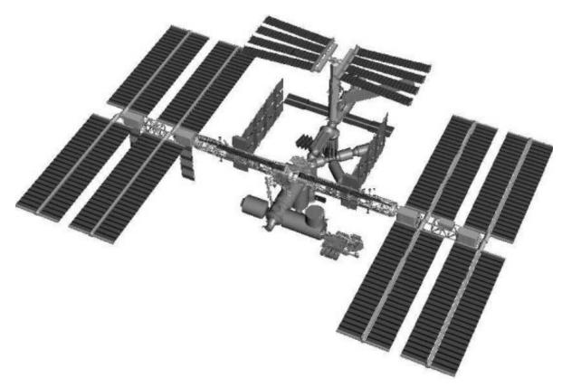
ISS Assembly complete 2005 Wingspan - 365 feet, 108 meters Length - 262 feet, 80 meters Mass - one million pounds, 454,000 kilograms Crew size - up to seven Laboratories - six
