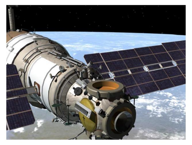
On the next ground station pass, controllers will reconfigure the module's on-board attitude sensors, activate it star tracker, and test the ability of a new communications system to relay information to Russian ground controllers
