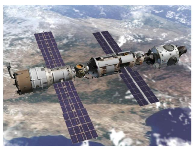
With the Zarya module controlling, the station will chase and catch up to Zvezda. Ground commands through Zarya's automated rendezvous system, will slowly pull the station next to the module, and then capture Zvezda
