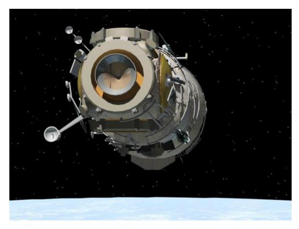
An automatic sequence of computer commands on Zvezda will order deployment of antennas for its Kurs rendezvous and docking system, and for the Lira communications system
