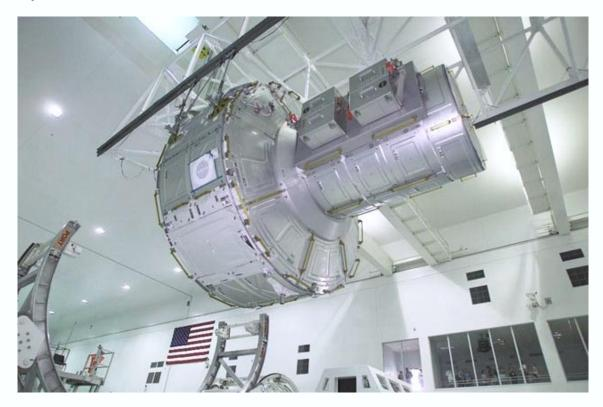
The airlock was shipped to the Kennedy Space Center last September aboard NASA's "Super Guppy" cargo aircraft. There it underwent leak testing and ground processing while multi-layer insulation and debris shields were installed on its exterior.
