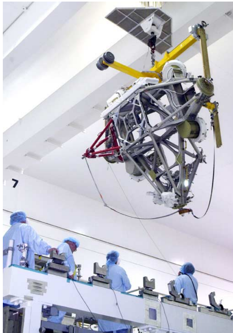
At Kennedy Space Center's Space Station Processing Facility, the Mobile Base System is hoisted to the weight and center of gravity stand
