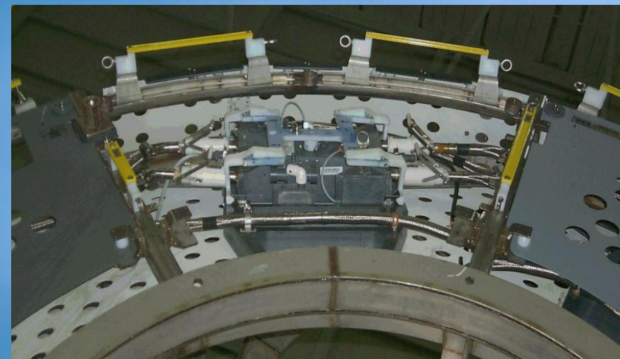
Small Hi-fi Mockup – Node 2 heat exchangers with functional interfaces
