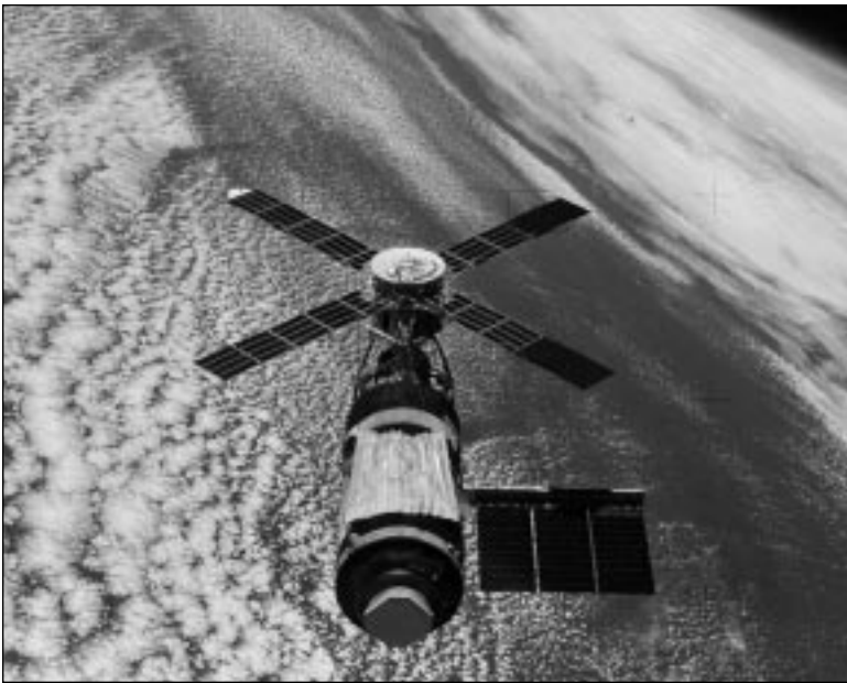
Mechanical failures during the May 14, 1973, launch landed Skylab in orbit overheated and starved for electricity. Astronaut EVAs saved the workshop and proved again the worth of humans in space. Skylab crews set new space endurance records and completed more experiments than originally scheduled, clearing the way for space experiments in the Shuttle era.
