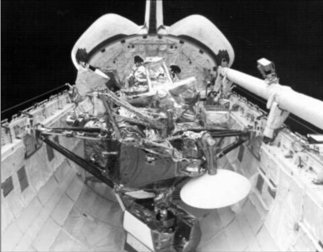
*This photograph of the Upper Atmosphere Research Satellite in the payload bay of the Earth-orbiting Shuttle Discovery shows the large size and versatility of the new space vehicle designed for near-Earth operations.*
