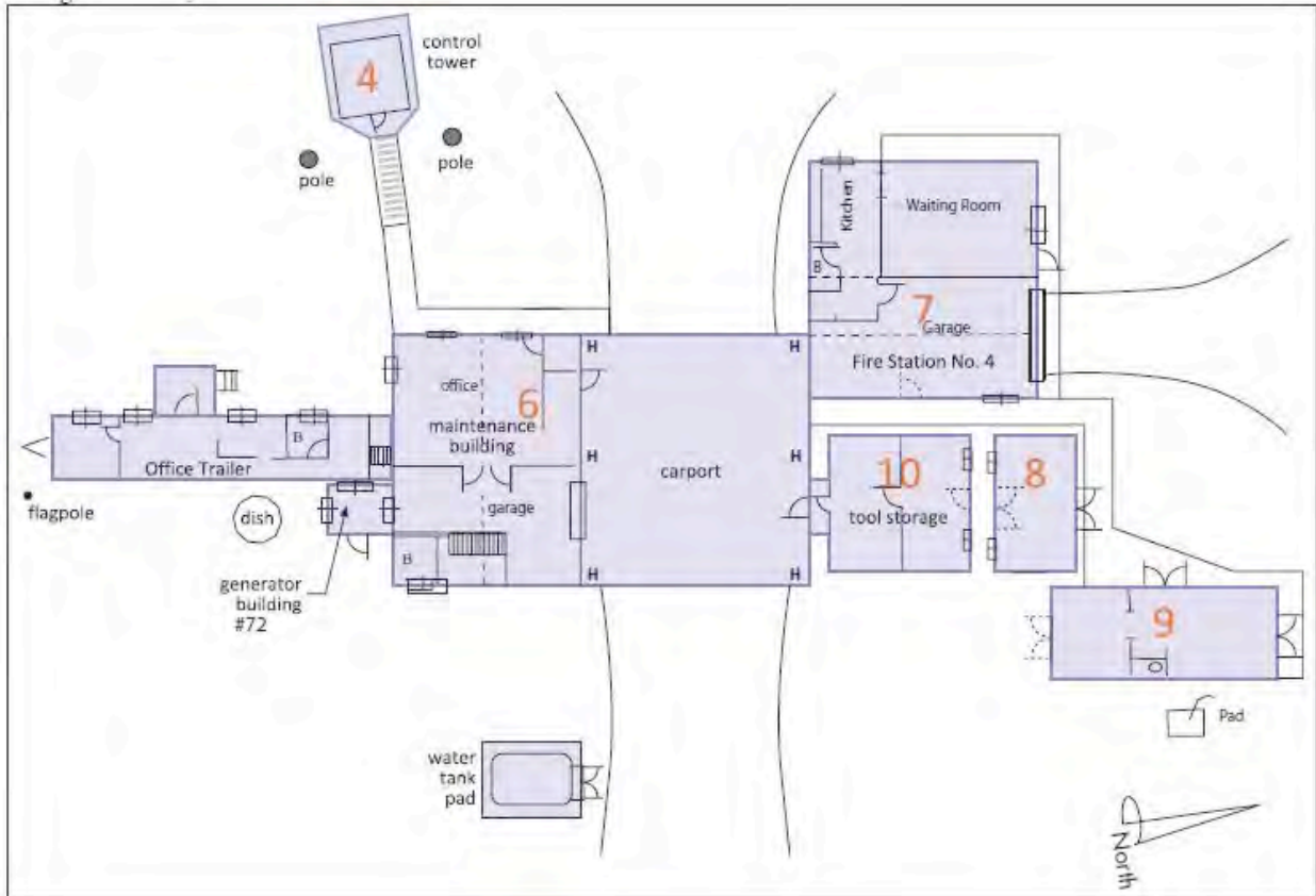
Figure 3. Plan map of the HUB complex in Area 1, including the Control Tower (4), HUB Maintenance Building (6), Fire Station No. 4 (7), NAVAIDS Storage Building (8), NAVAIDS Control Building (9), and HUB Tool Storage (10) (Drawn from not-to-scale site plan courtesy NASA WSTF).
