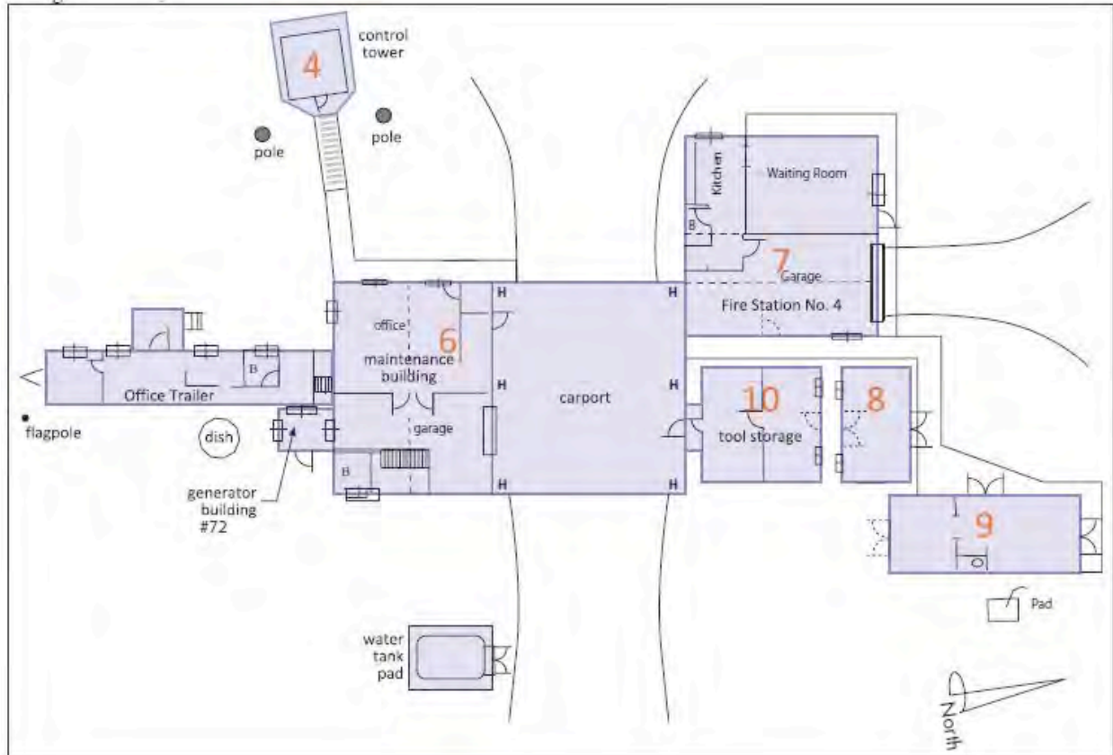
Figure 3. Map of the White Sands Space Harbor HUB complex showing the HUB Maintenance Building (#6). (Site Plan Source: NASA WSTF).
